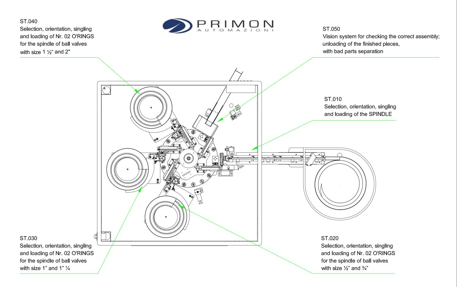
SPINDLE FOR BALL VALVES (of SIZE ½", ¾", 1",1"¼, 1"½ and 2") AUTOMATIC ASSEMBLY MACHINE
