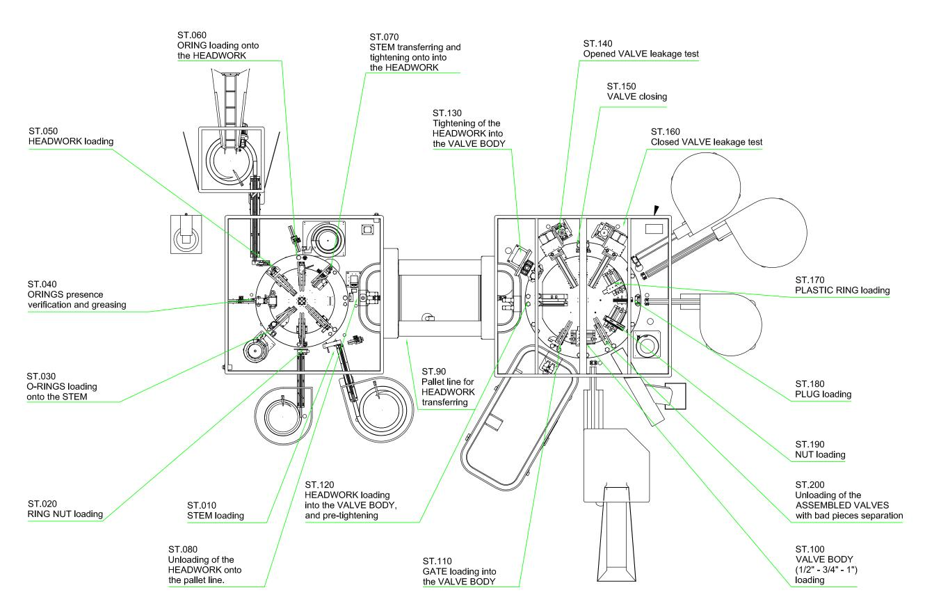
ASSEMBLING and TESTING MACHINE for GATE VALVES (1/2" - 3/4" - 1")
