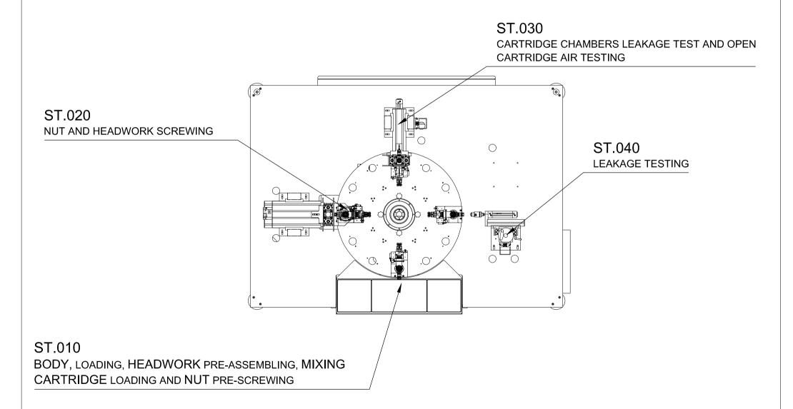
ASSEMBLING AND TESTING MACHINE FOR KITCHEN MIXER FAUCETS
